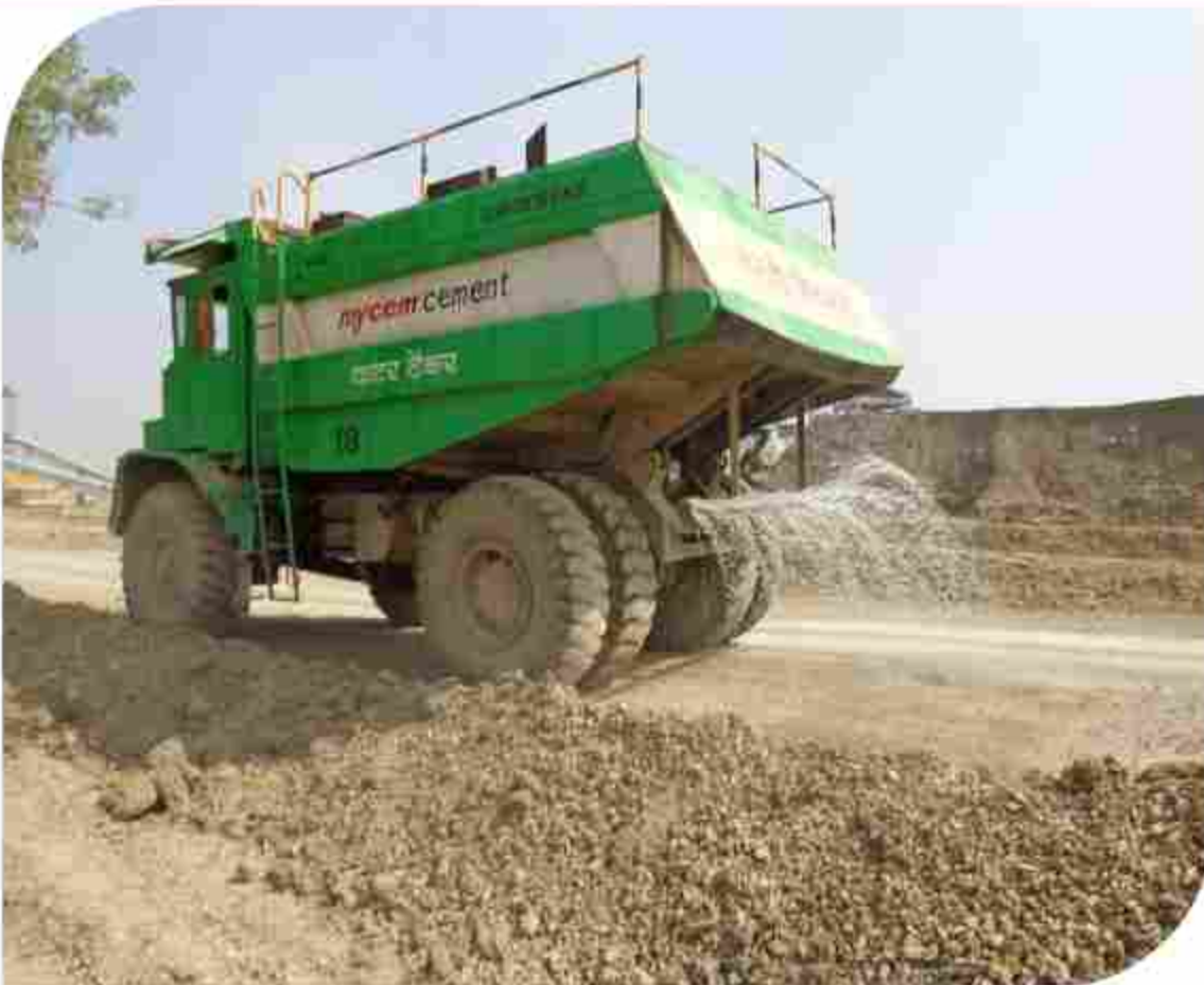
WATER SPRINKLING ON HAUL ROAD
